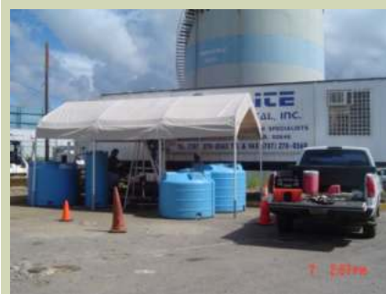
In-Situ Bio-Slurping System
