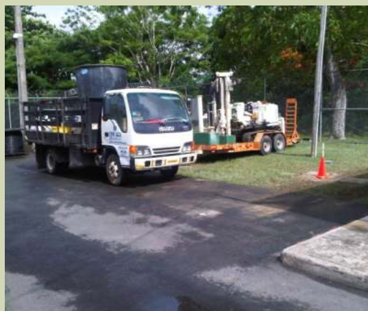
DPT/HSA Drilling Equipment
