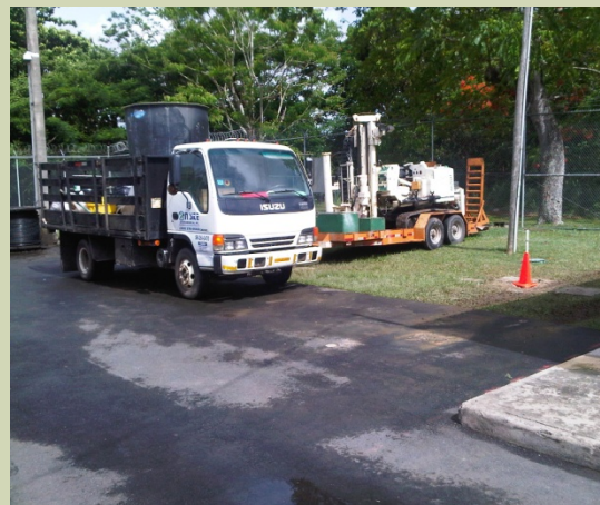
DPT/HSA Drilling Equipment
