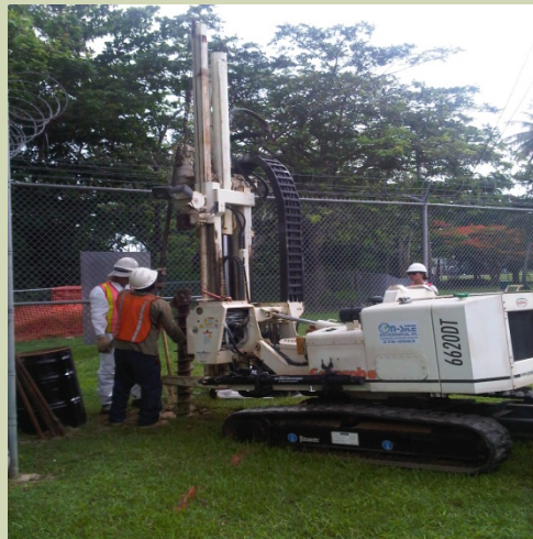
Soil & Groundwater DPT Sampling
