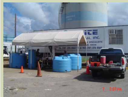
In-Situ Bio-Slurping System
